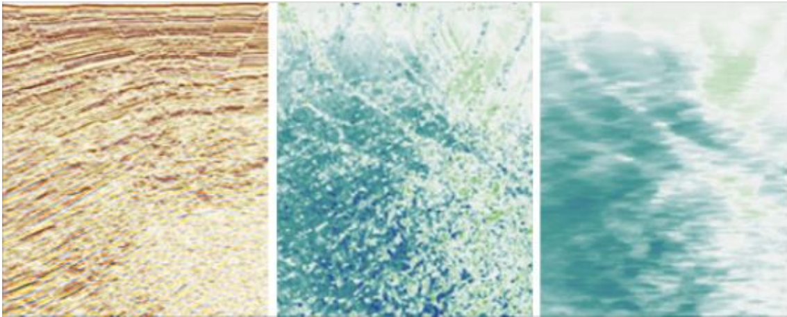
Examples of (left to right): Original Seismic (Full stack), Detailed Steering and Background Steering
