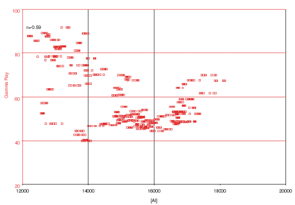
Figure 15. Cross-plots of gamma ray vs. acoustic impedance (left) and gamma ray vs. predicted gamma ray (right). Extraction is made from the well track of the blind test location mentioned in Figure 14. It is obvious that the neural network performs a better prediction of gamma ray than a linear correlation using acoustic impedance data alone.
