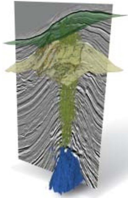
Fig. 6. Neural network enhanced seismic features: Salt dome (blue) and seismic chimneys (green) are detected by supervised neural networks; Alignment of chimneys and faults (dip-steered similarity) at a mapped horizon just above the drilling target show us that faults directly above the structure are leaking hence there is a high risk of drilling a breached trap (Heggland, 2002).
